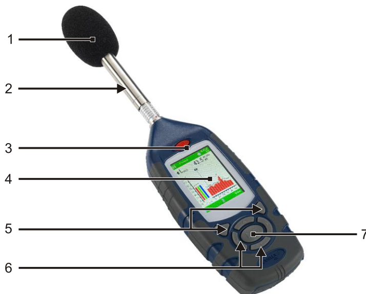
Figure 1. Main features of the CEL-63x sound level meter
